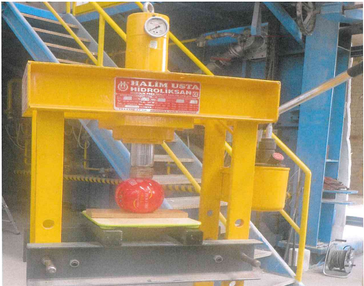
Photo 4: Pressure resistance test view.
