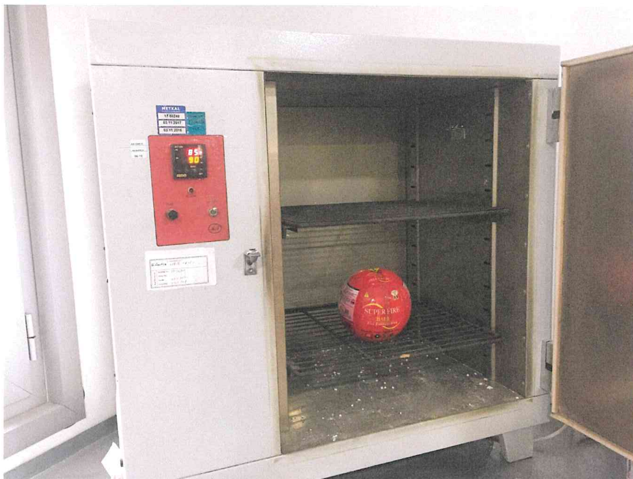
Photo 1: Thermal resistance test view.
