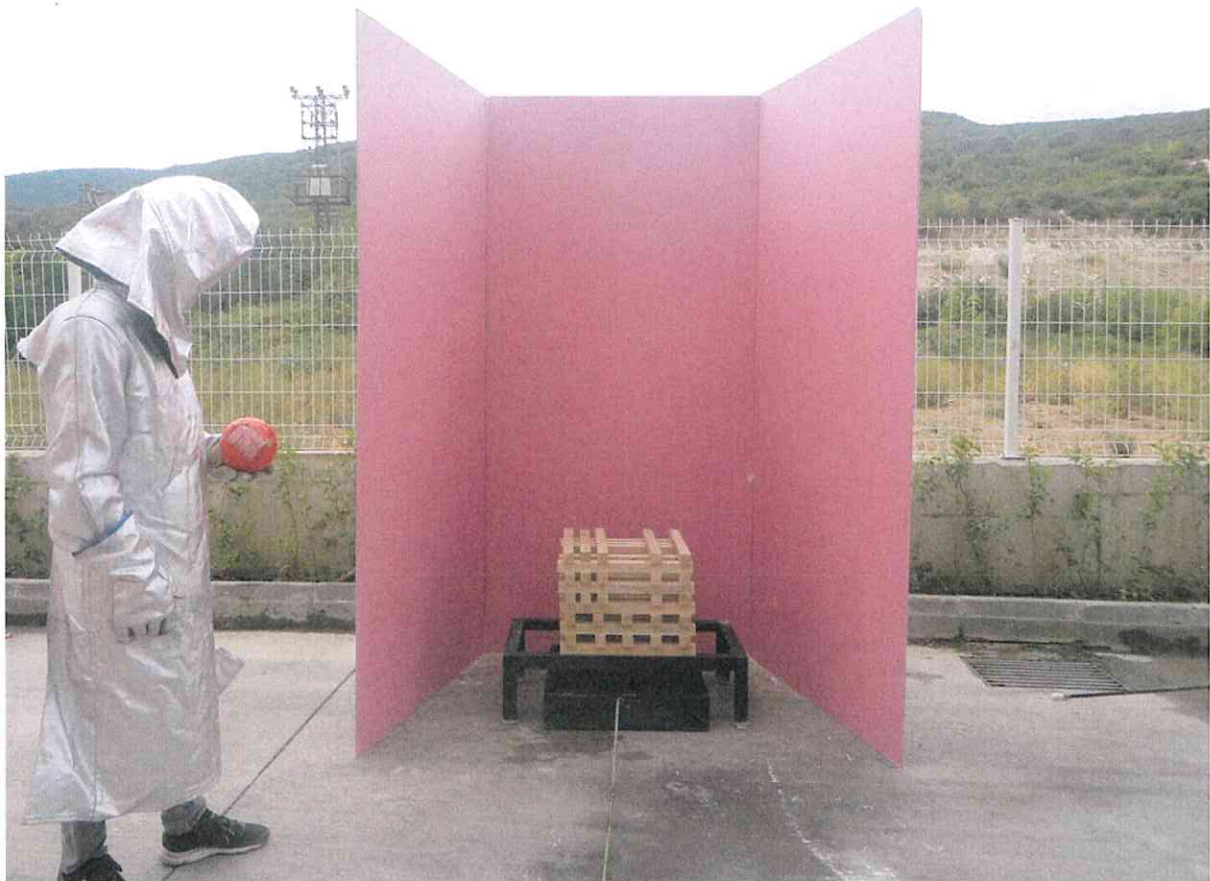
Photo 6: Before Class A fire test view.
